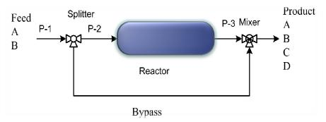
Chemical process of bypass similar to recycle
