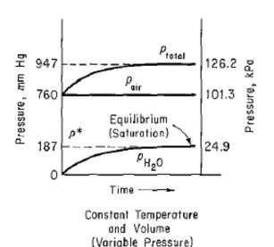
Change of partial and total pressures on vaporization of water into air at constant temperature
