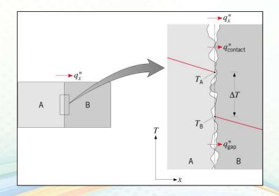
$$R_{t,c}^{\prime\prime} = \frac{T_A - T_B}{q_x^{\prime\prime}}$$
