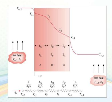
$$q_{x} = \frac{\left(T_{\infty,1} - T_{\infty,4}\right)}{\left[(1/h_{1}A) + (L_{A}/k_{A}A) + (L_{B}/k_{B}A) + (L_{C}/k_{C}A) + (1/h_{4}A)\right]}$$
