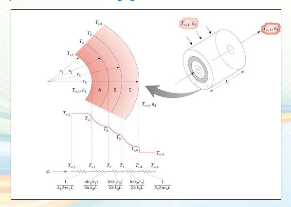
$$q_r = \frac{T_{\infty,1} - T_{\infty,4}}{R_{tot}} = UA(T_{\infty,1} - T_{\infty,4})$$
