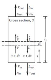
➤ Integrate from the top of the column down to the cross-section A-A:
