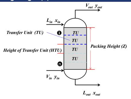
Packing Height (Z) = height of transfer unit (HTU) × number of transfer units (NTU)
