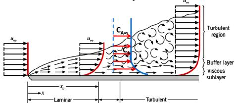
Three regions of mass transfer can be visualized. In the first, which is adjacent to the surface, a thin viscous sublayer film is present. Most of the mass transfer occurs by molecular diffusion, since few or no eddies are present. A large concentration drop occurs across this film as a result of the slow diffusion rate.
