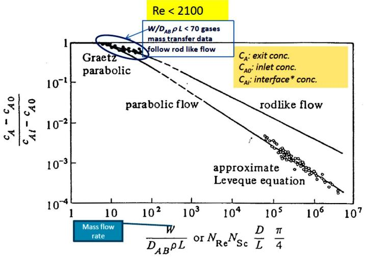
Data for diffusion in a fluid in streamline flow inside a pipe: filled circles, vaporization data; open circls, dissolving-solids data
