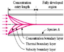
The development of the velocity, thermal, and concentration boundary layers in internal flow.
