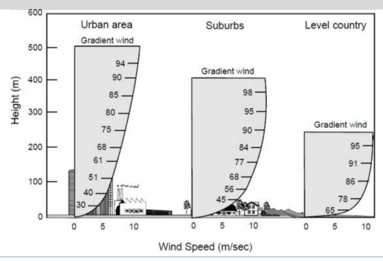
Examples of variation of wind with height over different surface roughness elements (Figures are percentages of gradient wind.) **Source: Turner 1970.**
