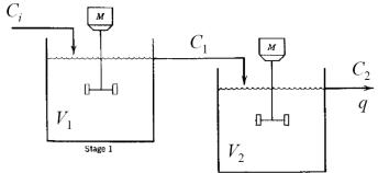
Parameters:  $V_1/q = 2 \text{ min}$ ,  $V_2/q = 1.5 \text{ min}$ .
