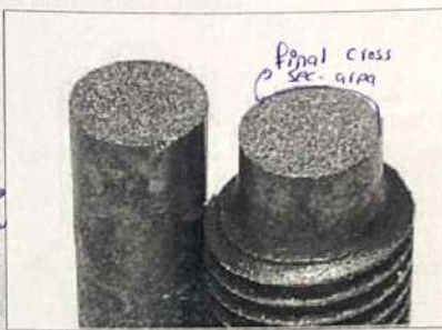
Brittle fracture in mild steel
