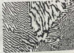
Micrograph of Pb-Sn Eutectic microstructure
