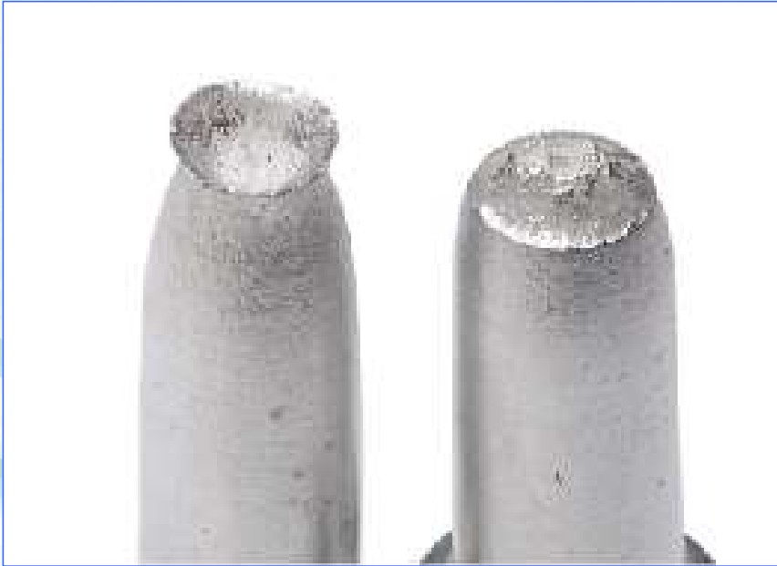
Cup-and-cone fracture in ductile Al
