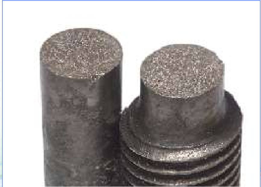
Brittle fracture in mild steel
