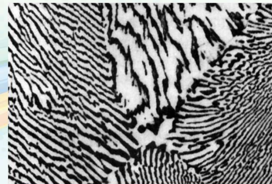
Micrograph of Pb-Sn Eutectic microstructure
