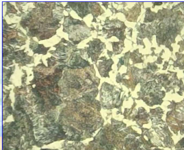
Perlite: ferrite and cementite
