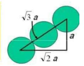
The higher coordination number and packing efficiency mean that this lattice uses space more efficiently than simple cubic.
