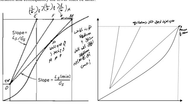
The minimum liquid that can be used corresponds to the slope of the operating line when touches the equilibrium curve (tangentially or intersection). At this ratio an infinite number plates (or height) will be required to obtain  $(X_{bottom})_{max}$ .
