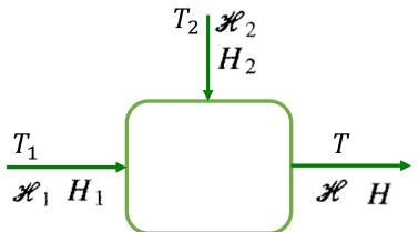
A mass balance on the dry gas, vapor, and enthalpy:
