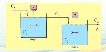
Parameters:  $V_1/q = 2 \text{ min}$ ,  $V_2/q = 1.5 \text{ min}$ .
