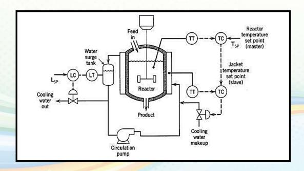
"Cascade Control of an exothermic chemical reactor"
