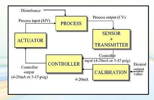
> The block diagram of feedback control system is:
