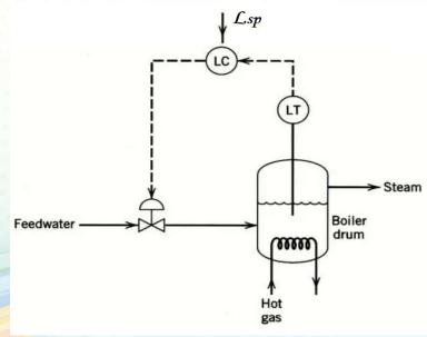
"Feedback control of liquid level in a boiler drum"
