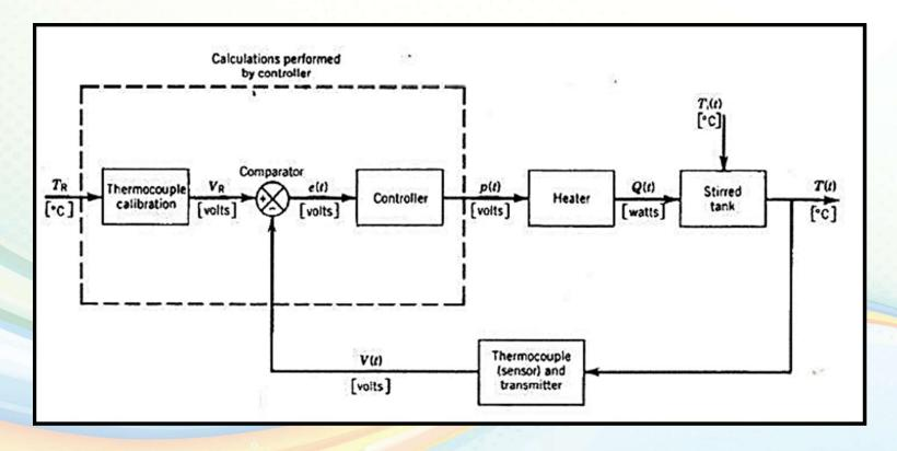
"Block diagram for temperature feedback control system"
