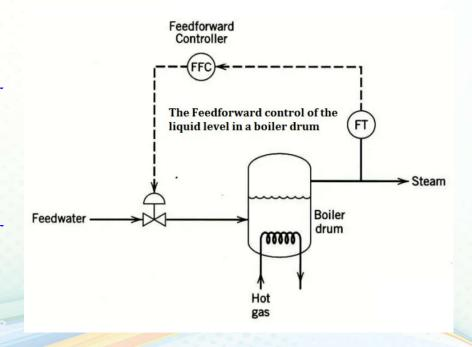
"Feedforward control of liquid level in a boiler drum"
