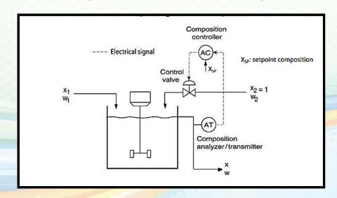
"Feedback control of composition (x) in Stirred-Tank blending system"
