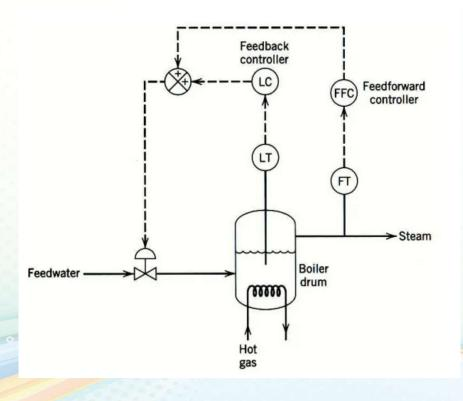
"Feedforward-feedback control of liquid level in a boiler drum"
