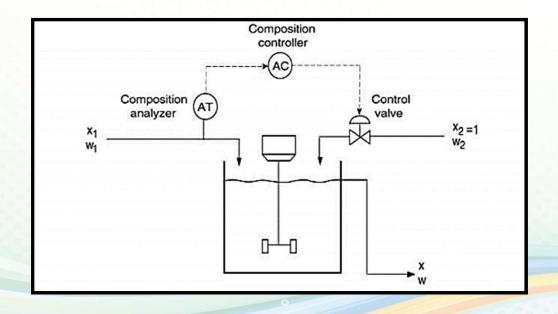
"Feedforward control of composition (x) in Stirred-Tank Blending System"
