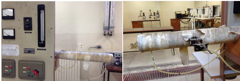
Figure (19): Pitot tube assembly front and rear views
