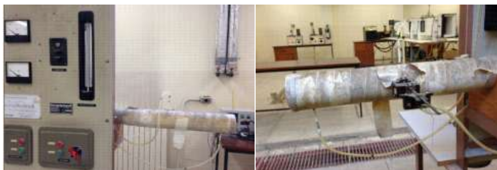
Figure (19): Pitot tube assembly front and rear views
