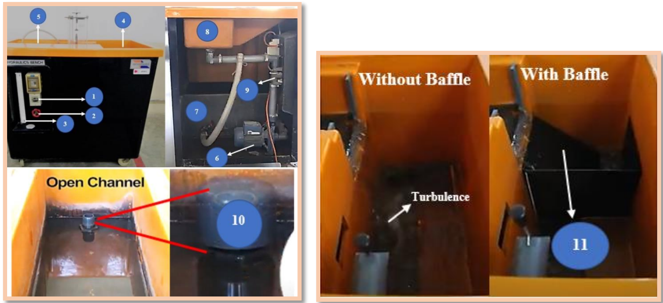
Illustration (2-B) : Digital Hydraulic Bench construction
