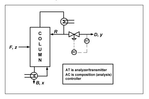
b) Feedforward Control: Measured variable: F Manipulated variable: D (shown), R or B
