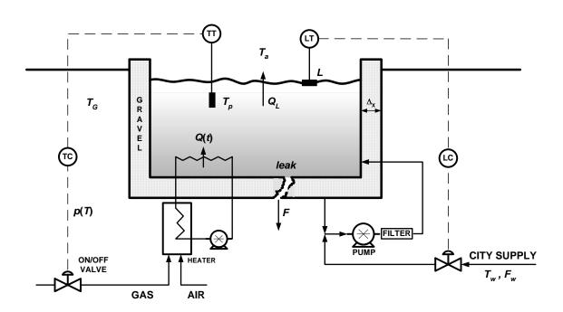
Outputs:  $T_p$ , L(level) Inputs: Q(t),  $F_w$ Disturbances:  $T_w$ ,  $T_a$
