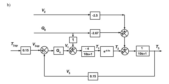
The control configuration in part a) will provide the better control. As is evident from the block diagrams above, the feedback loop contains, in addition to  $G_c$ , only a first-order process in part a), but a second-order-plus-time-delay process in part b). Hence the controlled variable responds faster to changes in the manipulated variable for part a).
