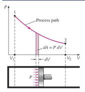
The area under the process curve on a P-V diagram represents the boundary
