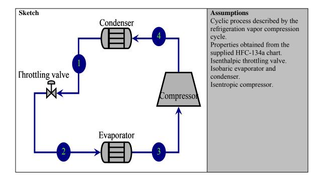
1. Supply the missing temperatures and pressures at each location in the provided table. Provide the vapor fraction if there are vapor-liquid mixtures.
