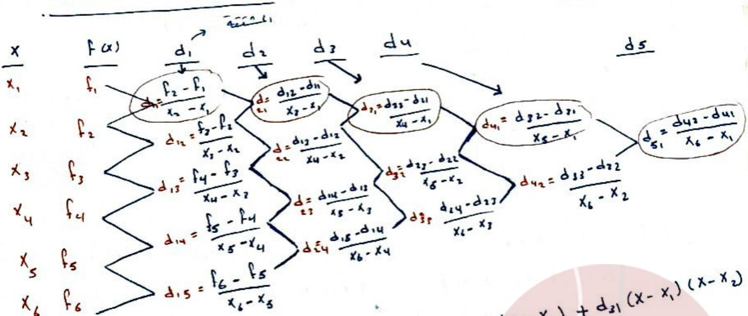
$$f(x) = f(x_0) + d_{11}(x - x_0) + d_{21}(x - x_1)(x - x_0) + d_{31}(x - x_2)(x - x_1)(x - x_0) \dots$$
