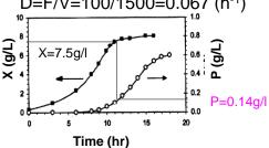
Product concentration can be increased by using multistage chemostats instead of single stage with the same total reactor working volume.
