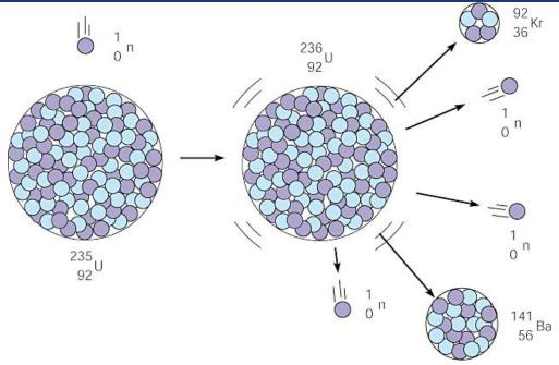
The fission reaction occurring when a neutron is absorbed by a uranium-235 nucleus. The deformed nucleus splits any number of ways into lighter nuclei, releasing neutrons in the process.
