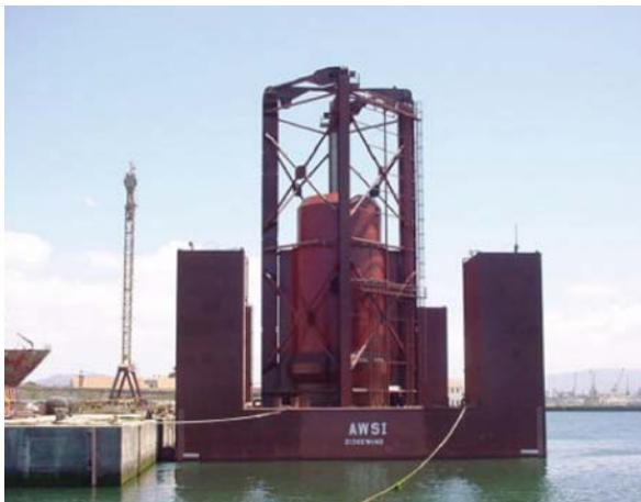
Fig. 9.17 Archimedes wave swing
