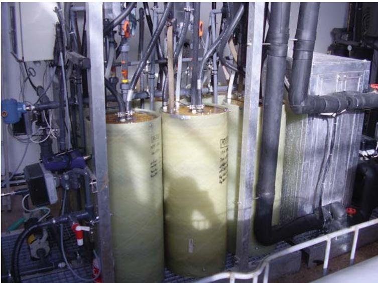
**Fig. 7.14** Desalination unit with five MD modules and heat exchanger (on the right)
