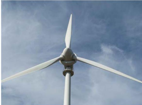
**Fig. 9.5** A gearless horizontal type 500 kW W/T
