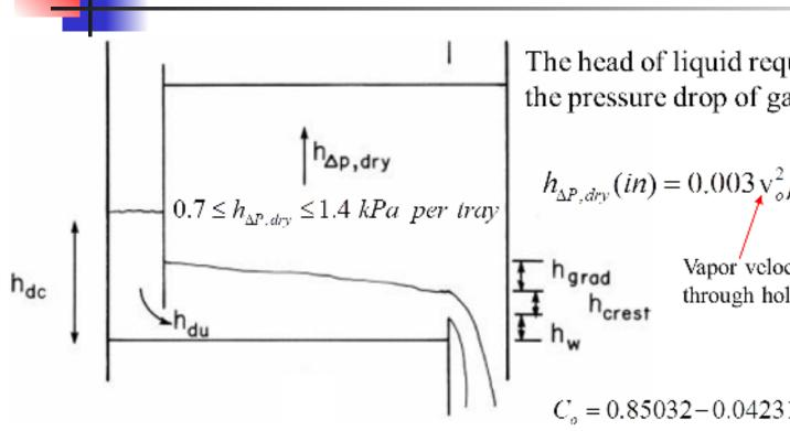
The head of liquid required to overcome the pressure drop of gas on dry tray  $(h_{\Delta P, dry})$ :
