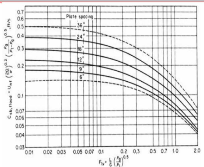
Plate spacing is the distance between the adjacent trays
