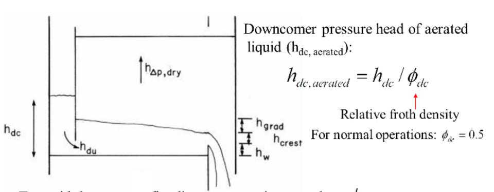
To avoid downcomer flooding, tray spacing must be  $> h_{dc,aerated}$ In normal operations, the tray spacing is  $> 2h_{dc}$
