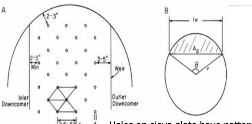
Holes on sieve plate have pattern to ensure even flow of vapor and liquid on the tray
