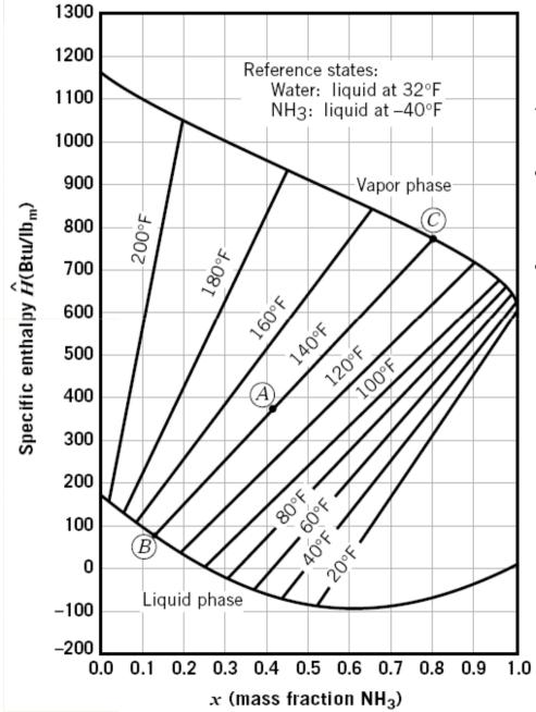
Fig. 8.5-2, p. 403, for liquid-vapor equilibria in the ammonia + water system at I atm pressure
