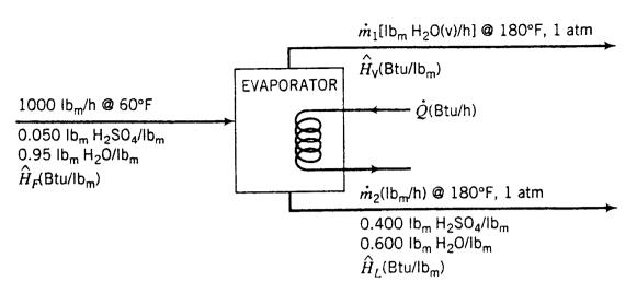
$$(0.050)(1000) \text{ lb}_{\text{m}}/\text{h} = 0.400 \dot{m}_2 \implies \dot{m}_2 = 125 \text{ lb}_{\text{m}}/\text{h}$$
