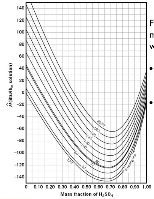
Fig. 8.5-1, p. 399, for liquid mixtures of sulfuric acid and water
