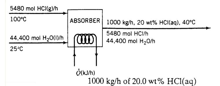
$$\dot{n}_{\text{HCl}} = \frac{1000 \text{ kg}}{\text{h}} \frac{0.200 \text{ kg HCl}}{\text{kg}} \frac{10^3 \text{ mol}}{36.5 \text{ kg HCl}} = 5480 \text{ mol HCl/h}$$
