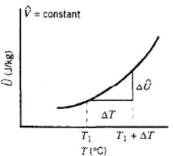
Since the plot of  $\hat{U}$  versus T is not generally a straight line,  $C_v$  (the slope of the curve) is a function of temperature.
