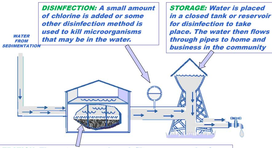
FILTRATION: The water passes through filters, some made of layers of sand, gravel, and charcoal that help remove smaller dissolved particles such as dust, bacteria, viruses, and chemicals.
