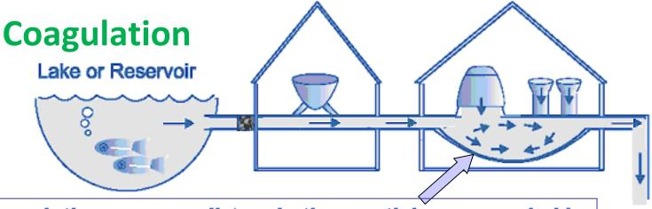
Coagulation removes dirt and other particles suspended in water. Alum and other chemicals are added to water to form tiny sticky particles called "floc" which attract the dirt particles. The combined weight of the dirt and the alums (floc) becomes heavy enough to sink to the bottom during sedimentation.
