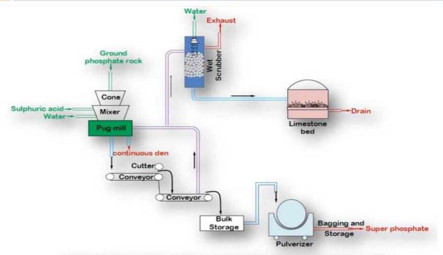
Figure: Manufacturing of Superphosphate by Continuous-den process
