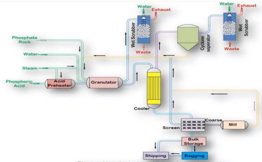
Figure: Manufacturing of Triple Superphosphate
