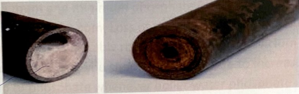
Boiler scale on water side
