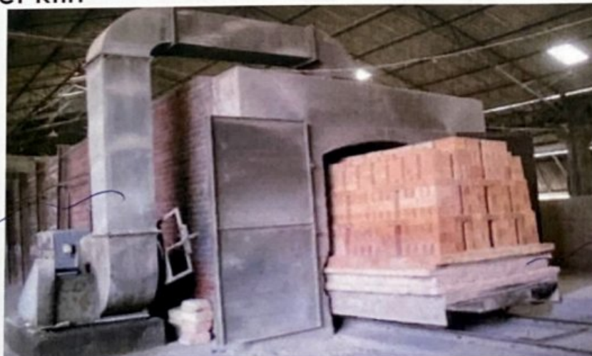
Tunnel Kiln Car loaded with Wares (Refractory Bricks) coming out of the Kiln after Firing
