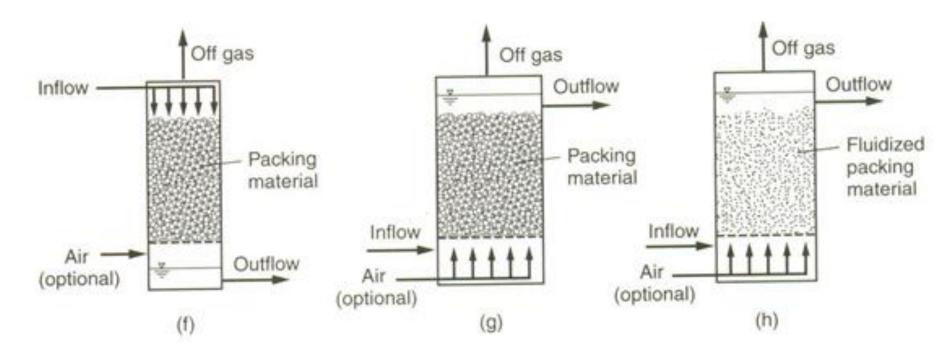
(f) packed-bed reactor, (g) packed-bed upflow reactor, and (h) expanded-bed upflow reactor.
