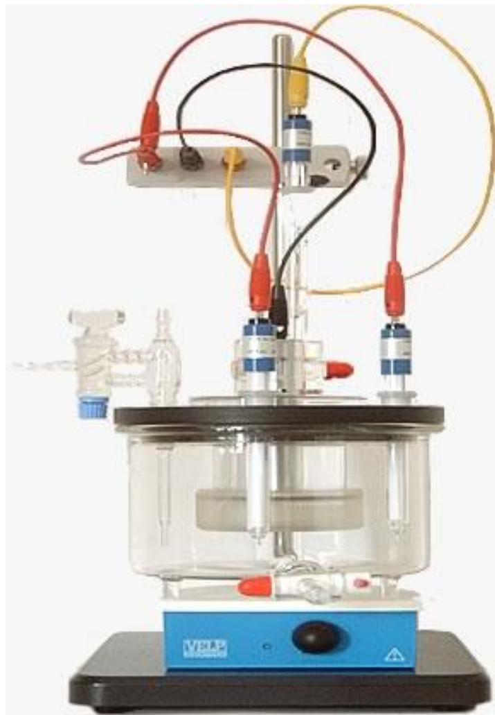
Figure (2.5): Cell apparatus for concentration polarization measurement
