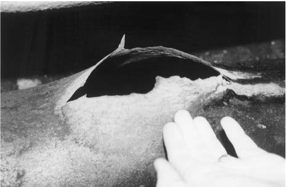
FIGURE 6-3 Close-up of the tube failure.
