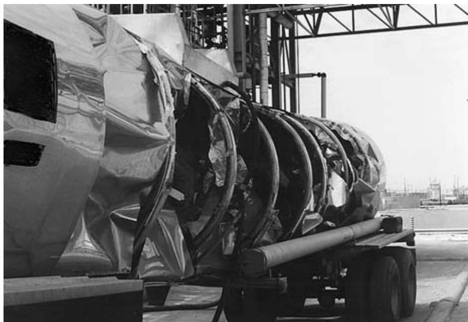
FIGURE 2-5 Close-up of tank failure and exposed ribs.
