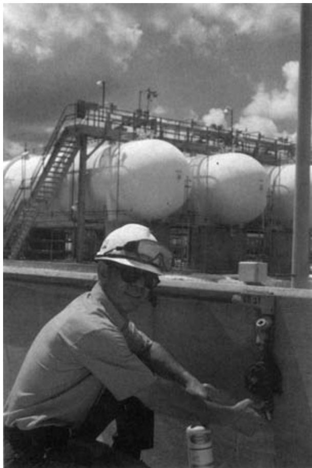
FIGURE 10–21 Prooftesting a flammable gas detector in a tank farm.
