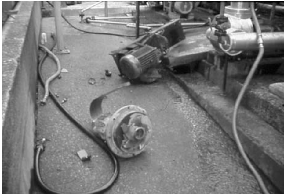
FIGURE 7-14 Pump base plate and motor as well as the position of the bearing housing with impeller document the explosion. Courtesy of Eastman Chemical Company.
