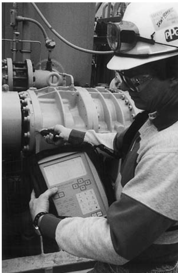
FIGURE 10-4 A close-up of a rotating machinery specialist with a vibration data acquisition module.
