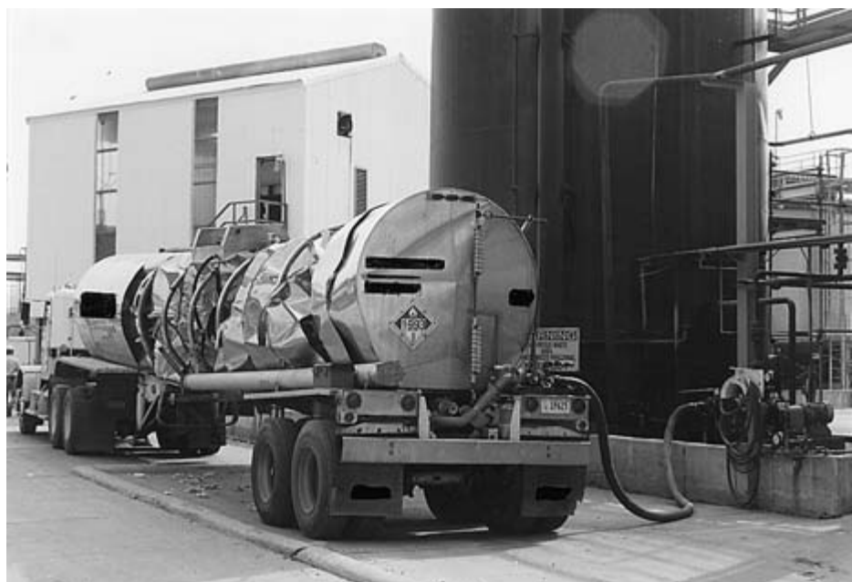
FIGURE 2-2 Collapsed tank truck with unloading hose connected.
