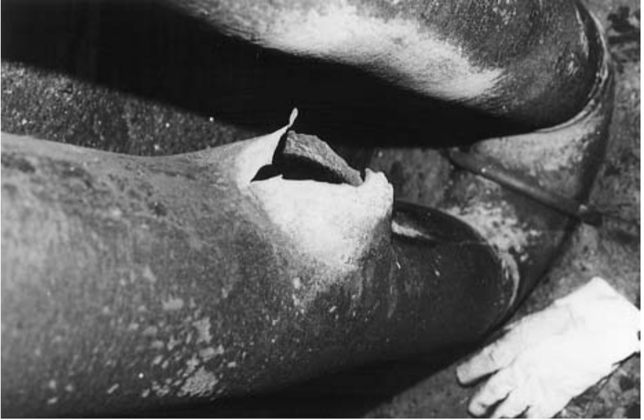
FIGURE 6-2 Tube rupture in a fired heater.
