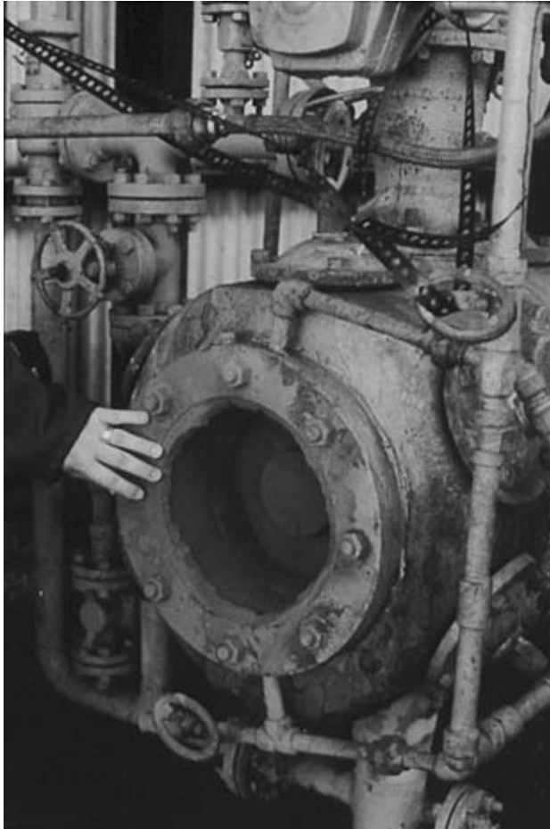
FIGURE 7-2 Close-up of ruptured water jacket on compressor.
