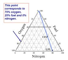
If 3 mol  $O_2$  is required to burn 1 mol  $C_2H_4$ , the stoichiometric concentration  $C_{st}$  in pure oxygen is 75%  $O_2$ , 25%  $C_2H_4$ .
