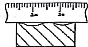
Figure 3.4 Gap between the workpiece and the Rule means the workpiece edge is NOT FLAT
