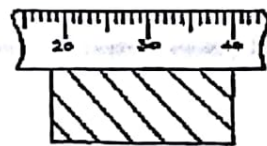
Figure 3.3 No gap between the workpiece and Rule means the workpiece edge is FLAT
