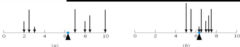
Figure 3-5 A probability distribution can be viewed as a loading with the mean equal to the balance point. Parts (a) and (b) illustrate equal means, but Part (a) illustrates a larger variance.
