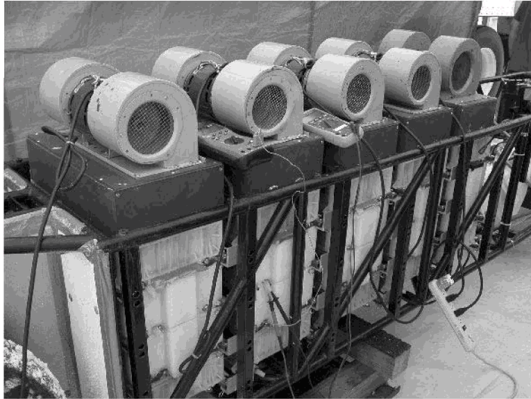
Figure 1.14 Battery pack (with cooling fans, used during charging and after a run)/Photo by Giorgio Rizzoni
