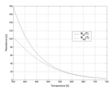
In the above plot, the solid line is for the thermistor alone; the dashed line is for the thermistor-resistor combination.
