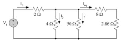
We can apply KVL and KCL to the above circuit:
