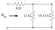
Then, we can combine the two parallel resistors, namely the 12  $\Omega$  resistor and 19.33  $\Omega$  resistor:
