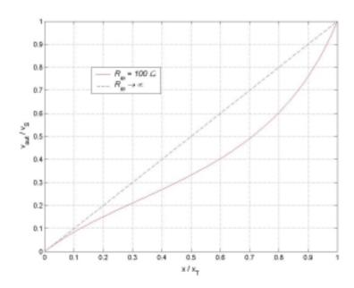
In the above plot, the solid line is for  $R_{\scriptscriptstyle m}=100\,\Omega$  ; the dashed line is for  $R_{\scriptscriptstyle m}\to\infty$  .
