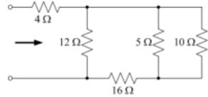
Then, we can combine the two parallel resistors, namely the 5  $\Omega$  resistor and 10  $\Omega$  resistor:
