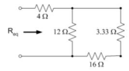
Then, we can combine the two resistors in series, namely the 3.33  $\Omega$  and the 16  $\Omega$  resistor:
