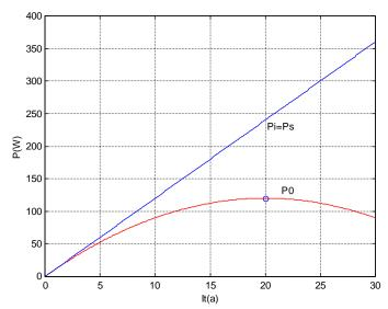
Note that the power supplied to the circuit is maximum when
