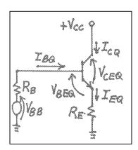
Redraw the circuit using the Thèvenin equivalent. The "DC blocking" or "AC coupling" capacitors act as open circuits for DC; therefore, the signal source and load can be neglected since
