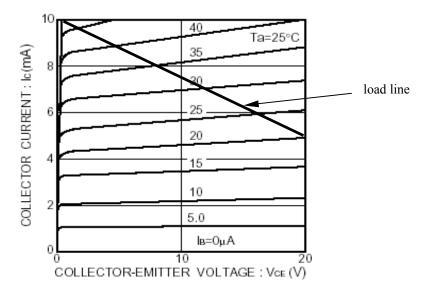
The operating point is at the intersection of the load line and the  $I_B=20\mu\mathrm{A}$  line of the characteristic. Therefore,  $I_{CQ}\approx5\,\mathrm{mA}$  and  $V_{CEQ}\approx20\,\mathrm{V}$ .
