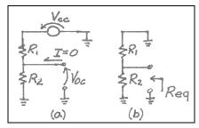
Note that  $V_{CC}$  must remain in the circuit because it supplies current to other parts of the circuit:
