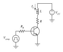
$$I_C = \frac{V_{CC} - V_{CEsat}}{R} = \frac{13 - 1}{12} = 1 \text{ A}$$
