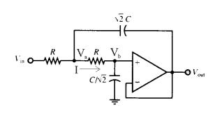
$$V_{a} = RI + V_{b} = R \left( j\omega \frac{C}{\sqrt{2}} V_{out} \right) + V_{out} = \left( 1 + j \frac{\omega RC}{\sqrt{2}} \right) V_{out}$$
