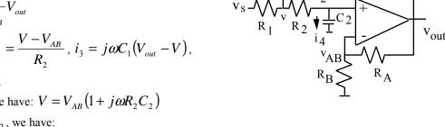
$$V_{out}\left(-j\omega C_{1} + \frac{R_{B}}{R_{A} + R_{B}}\left(\left(j\omega C_{1} + \frac{1}{R_{1}} + \frac{1}{R_{2}}\right)(1 + j\omega R_{2}C_{2})\right) - \frac{1}{R_{2}}\right) = \frac{V_{s}}{R_{1}}$$
