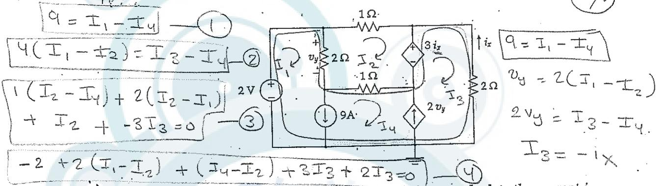
Q2. [18 points] Use superposition in the circuit below to calculate the current  $i$ . **IMPORTANT:** During your solution, you can only use current division, voltage division, Ohm's law, KCL and KVL, parallel and series combinations.
