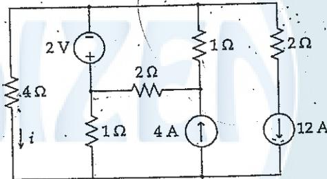
Q3. [18 points] Use source transformation in the circuit below to find the value of the voltage  $v_o$  given that  $i = 2$  A.
