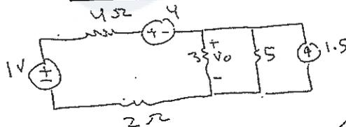
(2Ω, 4Ω) series  $\Rightarrow R_{eq} = 6 \Omega$
