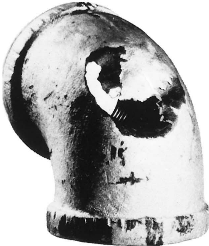
FIGURE 17.11 Impingement failure of an elbow that was part of a steam condensate line. (Photograph courtesy of Mars G. Fontana. From M. G. Fontana, Corrosion Engineering , 3rd edition. Copyright © 1986 by McGraw-Hill Book Company. Reproduced with permission.)
