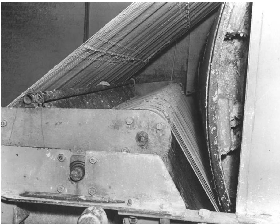
Figure 7.20. String discharge mechanism on a filter handling silica gel
