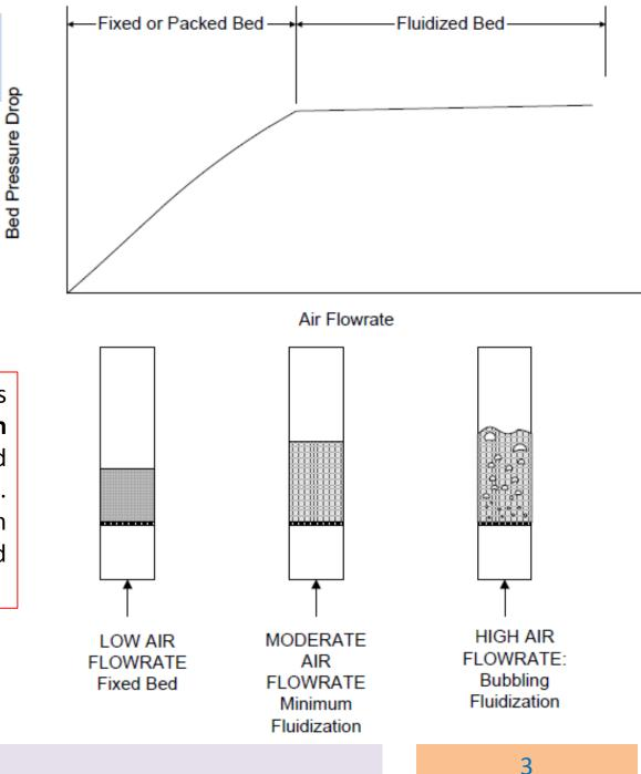
As shown in the figure, at gas flowrates less than the **fluidization velocity**, the bed is a fixed bed and there is no movement of particles. At flowrates above minimum fluidization the bed expands and bubbles appear.
