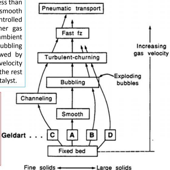
**Group C** cohesive, or very fine powders. Normal fluidization is difficult for these solids because of interparticle forces that are greater than those resulting from the action of the gas on the particles. In small diameter beds these particles form a plug of solids that rises upward. powders - very fine, cohesive powders which are incapable of fluidization in the strict sense. Examples: Face powder, flour, and starch.
