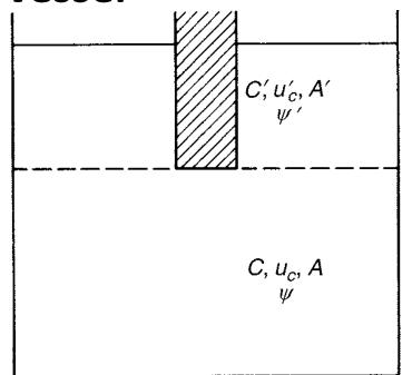
Sedimentation in partially obstructed vessel
