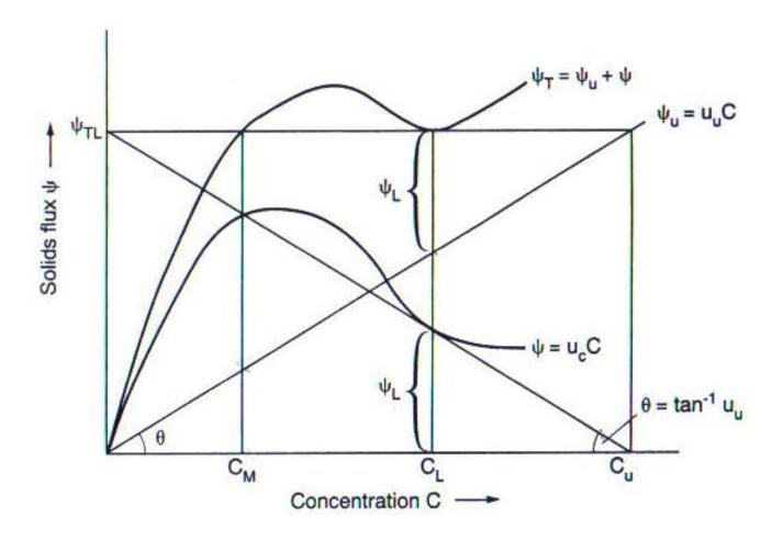
Fig. 5.13. Solids fluxes as functions of concentration and Yoshioka construction.
