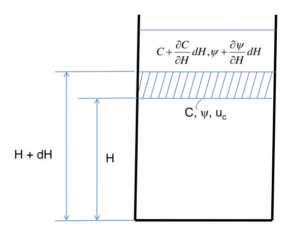
• In general,  $\psi$  = c u<sub>c</sub> Making a material balance between the height h and the height H+dH
