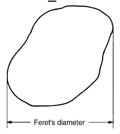
The mean distance apart of two parallel lines which are tangential to the particle in an arbitrarily fixed direction. Changing orientation will lead to a large number of Feret's diameter = 'Microscopy dimension'
