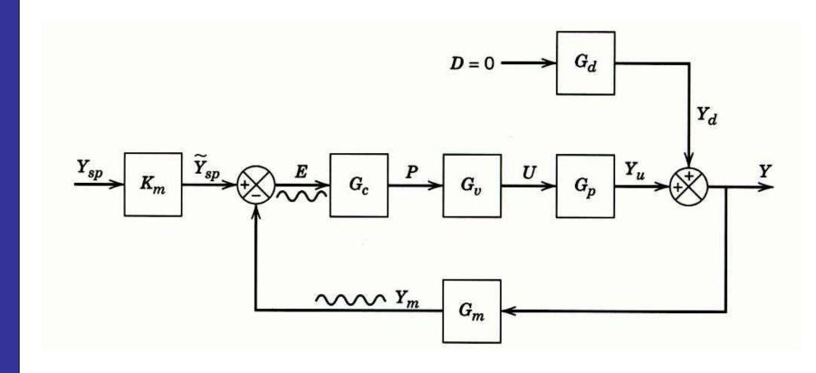
Figure 14.4 Sustained oscillation in a feedback control system.
