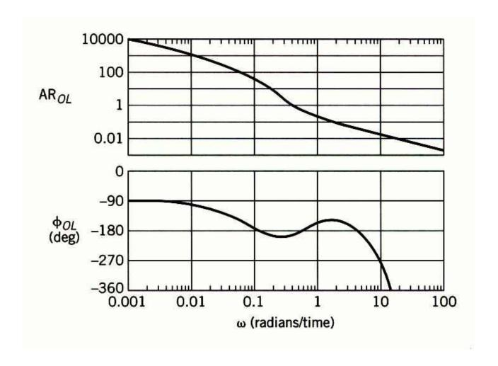
Figure 14.3 Bode plot exhibiting multiple critical frequencies.
