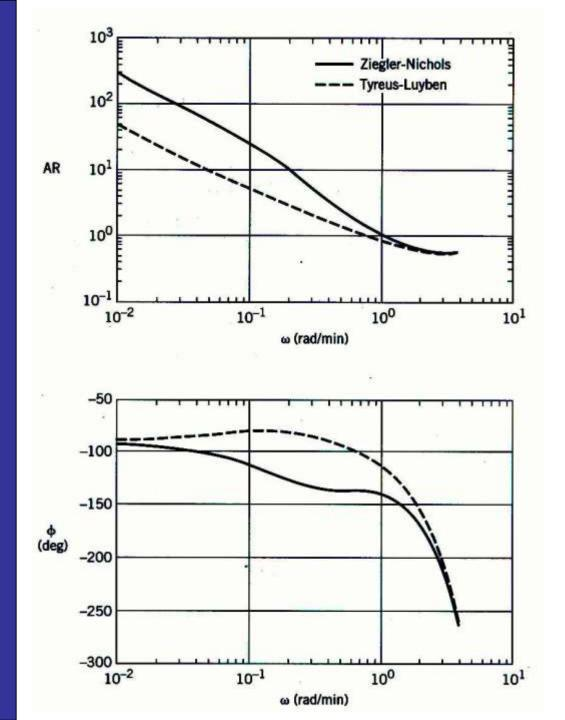
Figure 14.11 Comparison of  $G_{OL}$ Bode plots for Example 14.7.
