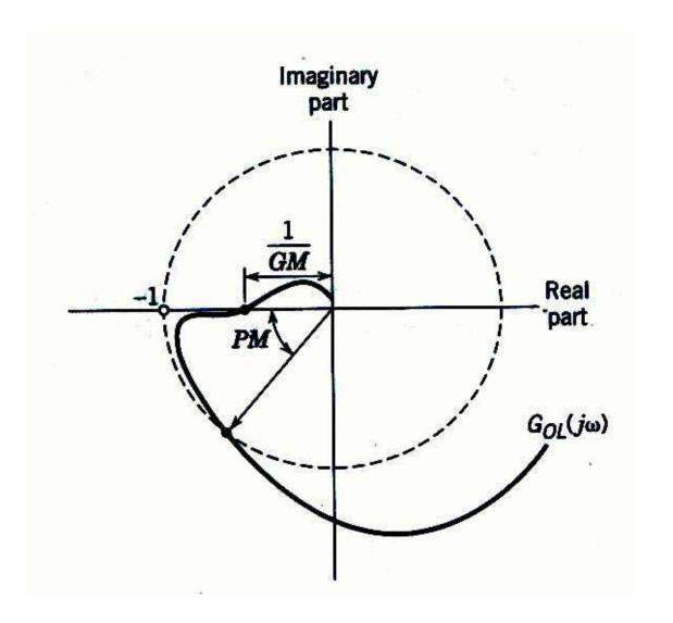
Figure 14.12 Nyquist plot where the gain and phase margins are misleading.
