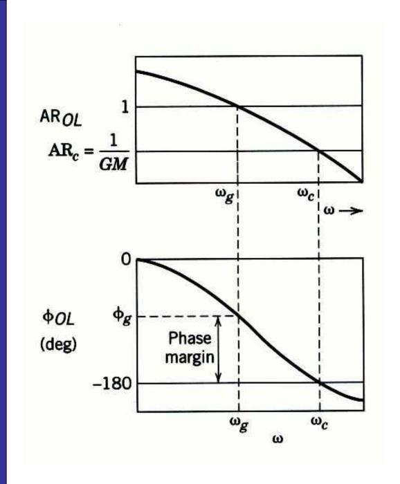
Figure 14.9 Gain and phase margins in Bode plot.
