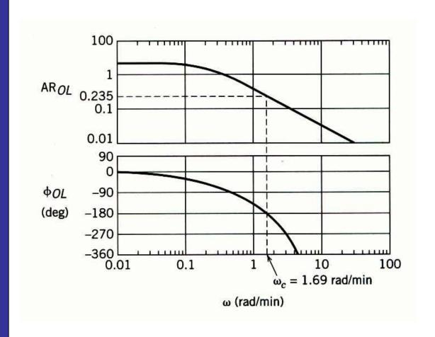
Figure 14.7 Bode plot for Example 14.6,  $K_c = 1$ . Figure 14.8 Nyquist plot for Example 14.6,  $K_c = 1.5K_{cu} = 6.38$ .
