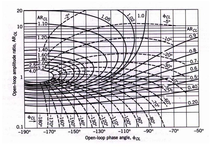
Figure 14.15 A Nichols chart. [The closed-loop amplitude ratio  $AR_{CL}$  (———) and phase angle  $\varphi_{CL}$  (———) are shown in families of curves.]
