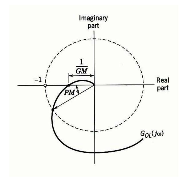
Figure 14.10 Gain and phase margins on a Nyquist plot.
